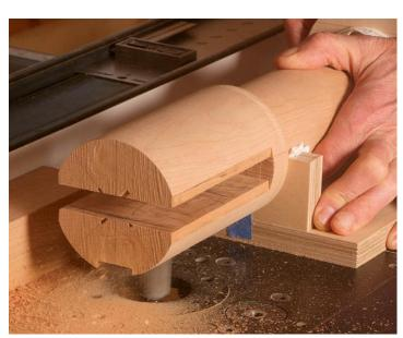
**Cut the groove for the stretcher.** With a U-shaped yoke screwed to the cradle serving as a clamp, use a router table to cut a stopped groove in the top end of the post (top). Square the rounded end left by the router bit with a chisel (right).
