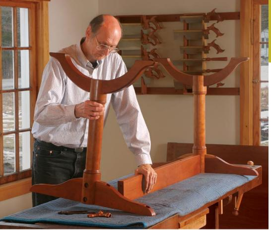
**Put it together.** After all the parts have been sanded and finished, it's finally time to put the table together. With the table parts upside down, slide the ends of the stretcher into the post grooves and slip the bed-bolt nuts into the mortises in the stretcher. Then, insert the bolts (top right).
