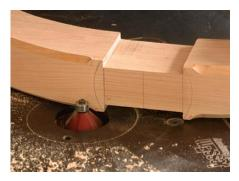
Rout chamfers. A chamfer bit in a router table is used to chamfer the top edges of the feet. Stop the cut ½ in. short of the dado.
