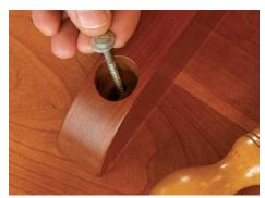
**Attach the top.** A screw and washer go into each counterbored hole in the braces. The slotted shank hole allows wood movement.
