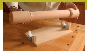
**Build a cradle.** Two saddles screwed to a base, ¾ in. thick by 8 in. wide by 12½ in. long, create a cradle for the post that simplifies a number of construction steps.
