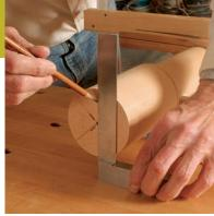
**Lay out the location of the notches.** With the cradle on a flat surface, use a square to mark a vertical centerline on each end of the post (left). Measure and mark the width of the notch, then use a square to scribe the notch depth (right).
