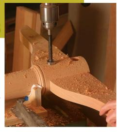
**Drill holes in the ends of the stretcher.** Add a trestle to the stretcher temporarily, then use a %-in.-dia. brad-point bit to extend the bed-bolt hole slightly into the end of the stretcher. After that, remove the trestle and drill deeper to complete the hole.
