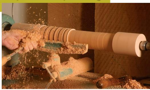
**Turn the blank.** Becksvoort turns a 35%-in.-sq. blank to 3½ in. dia., then makes a series of 23%-in.-dia. parting cuts along the midsection, checking the diameter with calipers. After that, with the parting cuts serving as guides, he reduces the entire midsection to 23% in. dia.
