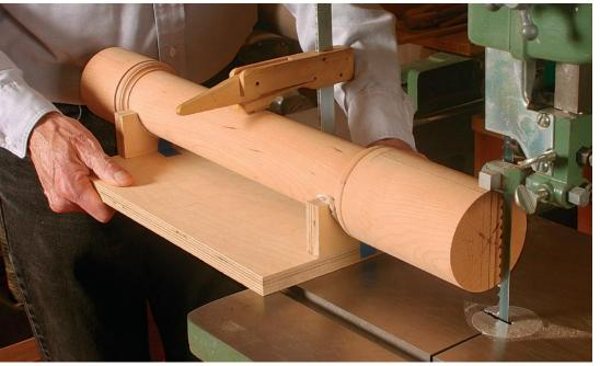
**Cut the two notches.** With the post securely clamped in the cradle, use a bandsaw to cut the notch on each end, following your layout lines by eye.
