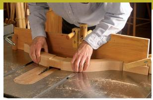
**Dado the legs and braces.** Cut a wide dado on each side of the brace and foot (above). Use the tablesaw miter gauge with a long auxiliary fence to support the parts during the cuts. A pair of stop blocks helps ensure that the ends of the dadoes end up perfectly aligned on both sides of the parts.
