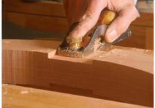
Dry-fit the parts. Check the fit of the posts to each dado (above). If too tight, use a rabbet plane (left) to trim the sides or bottom of the dado.
