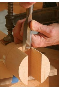
**Hand work.** Smooth the ends of the notches and the cheeks with a sharp chisel.
