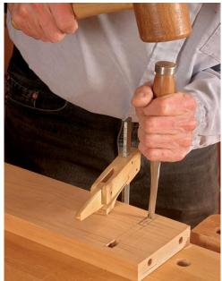
Lay out the location of the bed-bolt nuts. With a bed bolt in a stretcher hole serving as a guide (in case the hole isn't drilled perfectly square), mark the location of the bedbolt nut (above). Cut the mortises for the nuts (left) just deep enough to allow the bolt to thread into the nut.
